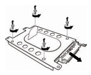
Figure 4-5 Removing the HDD connector
